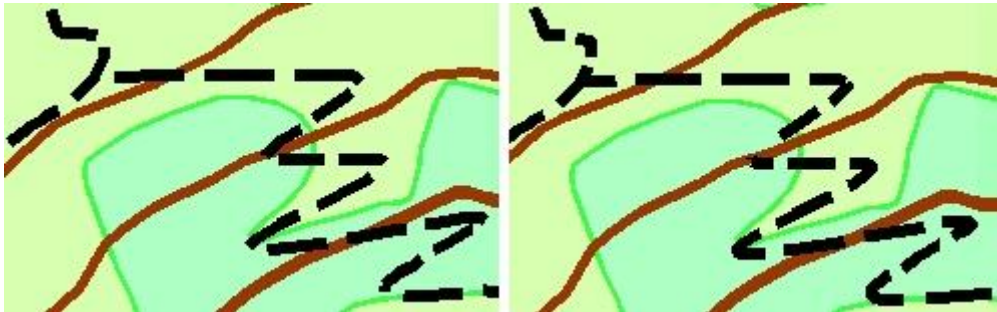
Figure 9: Automatic correction of unwanted gaps in dashed lines.
